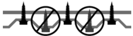
A one-corrugation side lap is necessary. If lapping panels end-to-end, make sure that water will flow over the lap, and use a 4 inch or greater overlap in these areas. Fasten in all the peak corrugations at end laps. Wait to install the side lap and end lap fasteners until subsequent sheets are installed.
